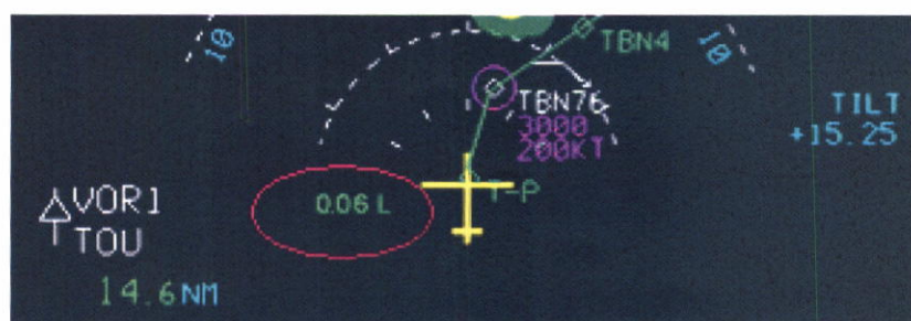
Figure 10.2: Lateral deviation displayed on a navigation (map) display
